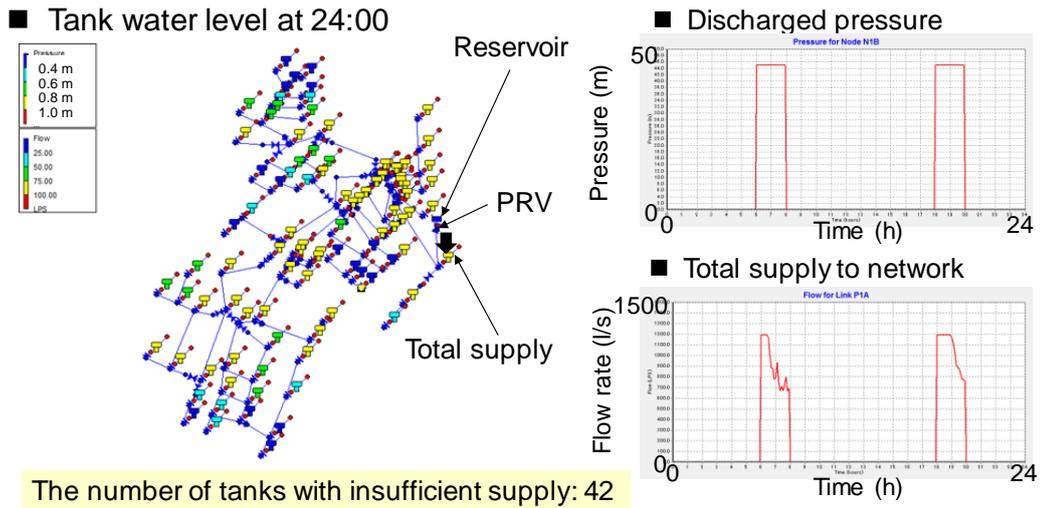
Figure 8 Tank water level at 24:00 in case 2
