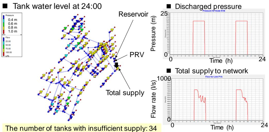
Figure 6 Tank water level at 24:00 in case 1
