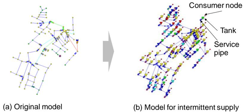
**Figure 2** Creation of hydraulic model for intermittent supply by conversion program
