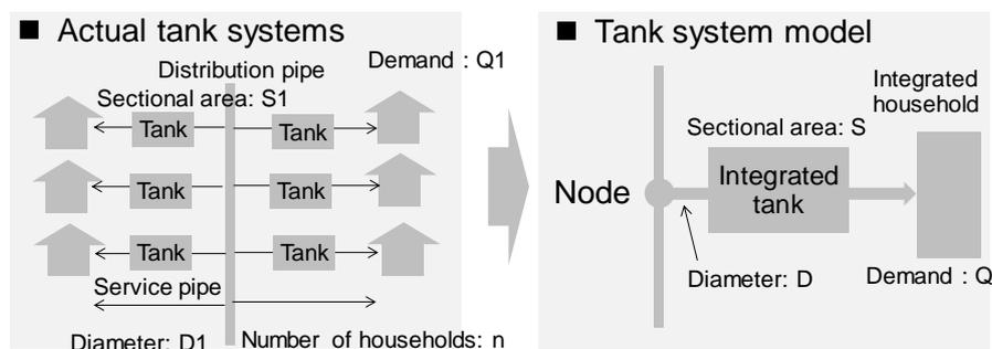
**Figure 1** Tank system model
