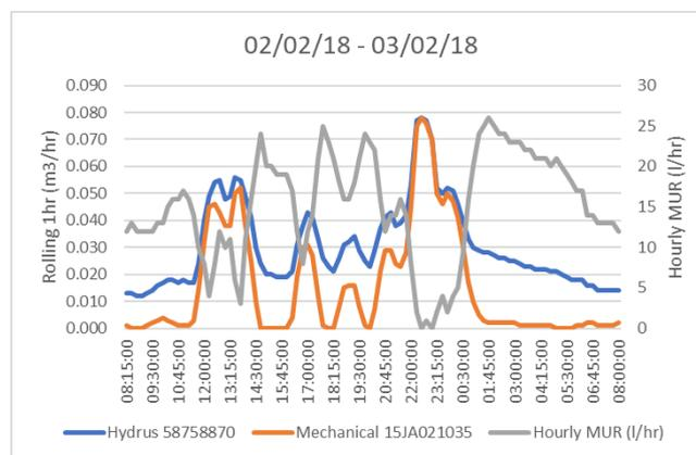
**Figure 6** 1hr rolling average trace for meter 15JA021035 and associated Hydrus with MUR expressed in l/hr
