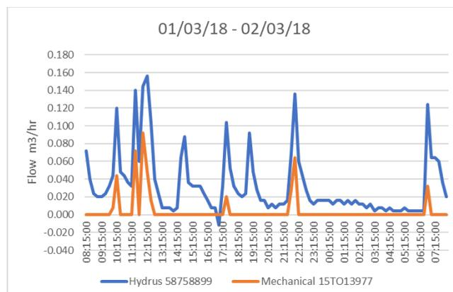
**Figure 4** Daily trace for meter 15TO13977 compared to associated Hydrus meter
