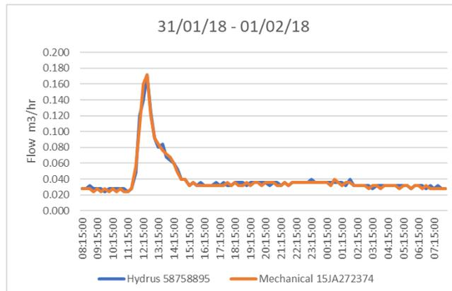
Figure 10 Trace of meter 15JA272374 showing presence of a leak on the property
