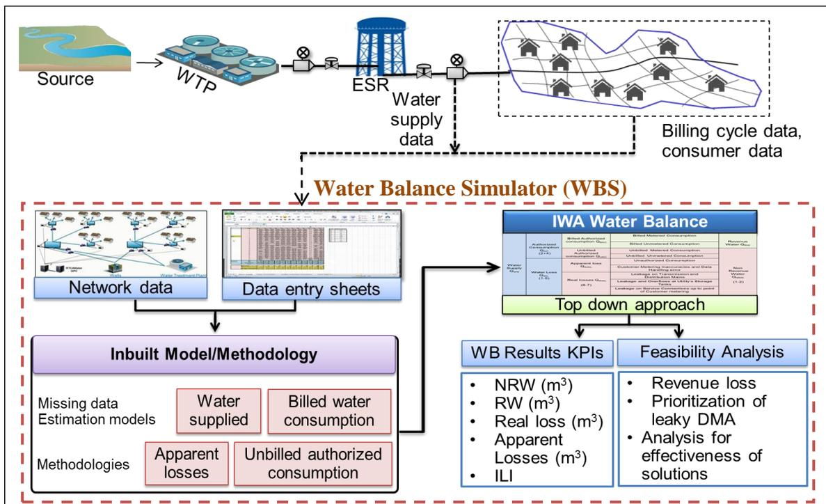
Figure 1 Structure of WBS (Water Balance Simulator)
